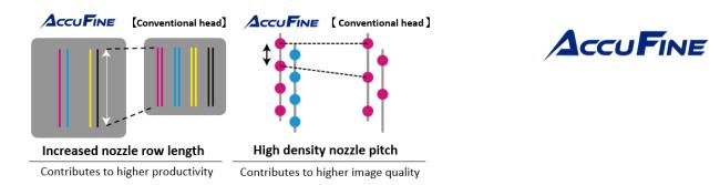
The new print effect "i-screen", created from MUTOH's "Intelligent Interweave" printing technology, optimizes the new print head "AccuFine". By arranging the dots in a way that takes into account how they look, this reduces banding for smoother print images.
