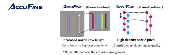
**The new print effect "i-screen"**, created from MUTOH's "Intelligent Interweave" printing technology, optimizes the new print head "AccuFine". By arranging the dots in a way that takes into account how they look, this reduces banding for smoother print images.
