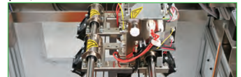
Two cooling fans are equipped at before and behind of each extruder.
