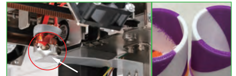
A shutter (white arrow) which covers up a waiting extruder (circled in red) reduces excrescence (right side of the photo).
